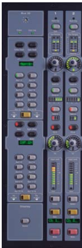
Encoder assignment switches and input channel strips
